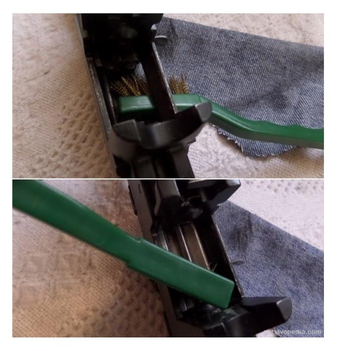
**Step 10** — Use Q-Tips soaked in gun cleaner to clean the bolt and receiver. Use dry Q-Tips to remove excess cleaner. Then use Q-Tips with gun lubricant to lube the bolt and the inside of the receiver. Use only a drop or two on the Q-Tip. Do not overdo it.
