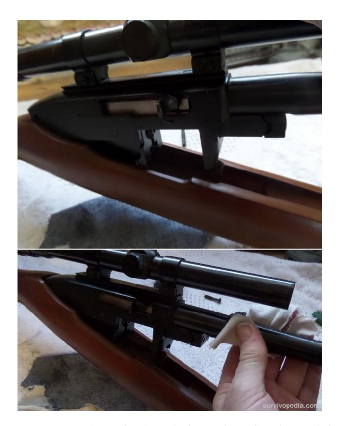
**Step 13** — After the barreled receiver has been lightly lubricated, assemble it back into the stock. Then insert and tighten the stock screw.
