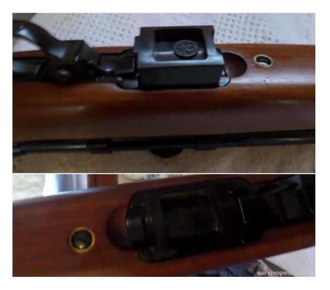
**Step 18** — After function testing the rifle wipe down the barrel and any other places that you touched on the rifle with a clean lubricated rag. This is to prevent the sweat in your finger tips from rusting any exposed parts of the rifle.
