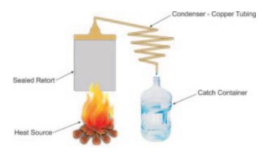
Perhaps the easiest way to build a still is to start out with a pressure cooker or pressure canner. This provides a sealed retort, with a single outlet; the one used to allow steam to escape, regulating the pressure in the pressure cooker. We would need to remove the normal pressure regulator from that point, drill the hole out and thread it for the attachment of a brass fitting, so that we could attach the condenser tubing to it.
