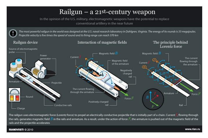
Once the projectile reaches the end of the rails, it is going so fast that it will continue on its path without using more energy from the power source. There are also newer designs that do not require a projectile. Newer rail guns being developed by the military can use pure energy as the "projectile". Typically, these guns fire as much as 33% faster than conventional explosive based guns.
