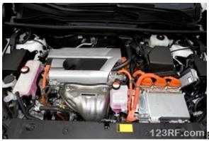
Be very careful when working on any part of a hybrid or electric vehicle because their internal systems have very high voltages that can easily kill you. If you must work on this type of vehicle, always consult with a mechanic certified to repair and adapt these vehicles.
