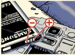
2: LOCATE the positive and negative terminals on the battery. Look for small gold plates on the bottom of the battery. The outermost plates are the positive and negative terminals.
