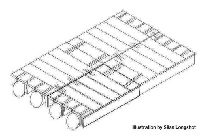
Since you may not be so lucky as to find the needed amount of barrels, you could tear apart sufficient numbers of pallets to fill underneath the ones intended to be the raft, with the amount of wood to get pretty good floatation. This would have to also be lashed in place, like the barrels, as shown here:
