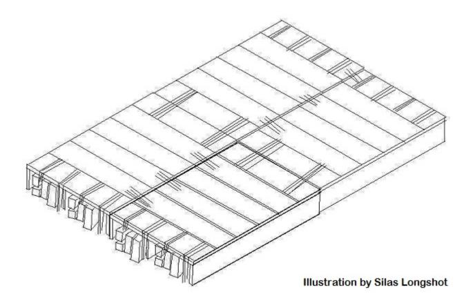
If you're lucky enough to find Styrofoam blocks of sufficient size to substitute for the barrels, the raft will be considerably lighter. If you find a massive pile of Styrofoam peanuts and heavy duty trash bags that you can empty out, you can bag up the foam equally into the bags assuming they're large and tough enough and of roughly equal size.
