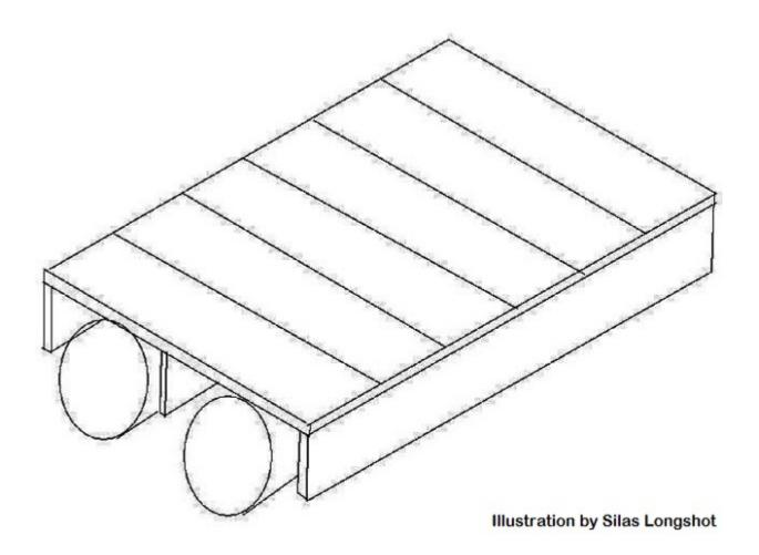
You will have to lash or bind the barrels to each pallet and each pallet to the other until you have a roughly square construction like so, with a barrel or two under each pallet. See the picture below for illustration. (These sketches are not to scale by any means, just a display of the concept.)
