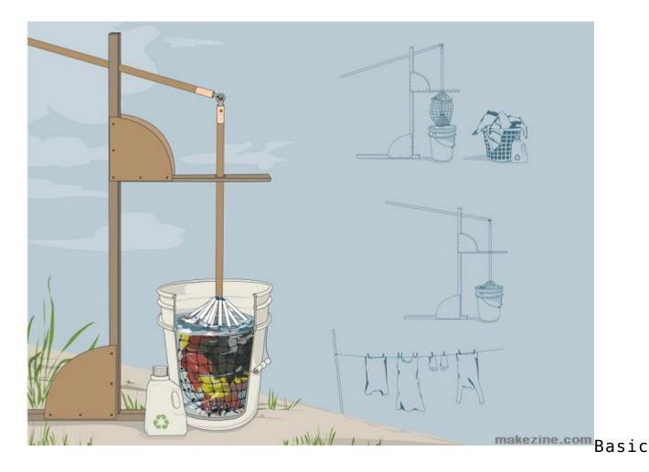
ally, this highly portable muscle-operated washing machine is made of three main components: the container itself, a net bag (this is designed to agitate the clothes while it holds/squeezes them) and the mechanism itself, which is a lever-driven shaft kept together by a wooden frame.
