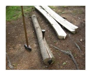
"This rough guide of How To Split Logs lengthwise using wedges to create lumber for building projects.
