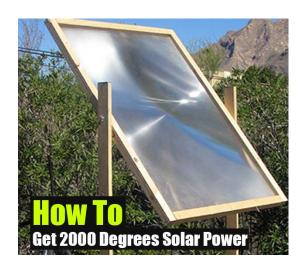
This is made from a simple lens called a Fresnel lens... These are commonly found in old rear projection big screen TVs ....
