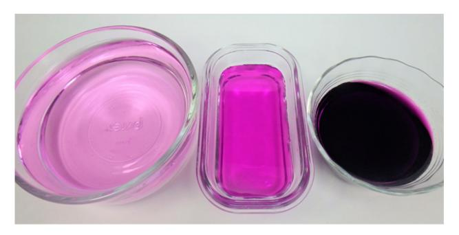
In the above photo, I have mixed three concentrations of KMnO4 in water. An amount of this chemical small enough to fit on the head of a tack is enough to treat dozens of gallons of drinking water or to create several liters of bright purple solution for signaling on snow. Put the solution in a water bladder with a squirt cap or place it in a plastic bag and make a small hole so you can develop just enough pressure to create large letters in the snow.
