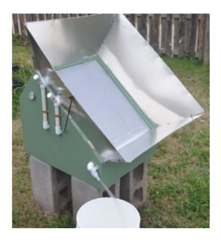
As you can see in this picture, the solar still looks more like a solar oven, than it does the previous still we looked at. The reflectors show on the still above are made of polished aluminum and increase the amount of sunlight entering the cabinet of the still, which is insulated and painted black on the inside, to facilitate absorbing the sunlight and converting it to heat.
