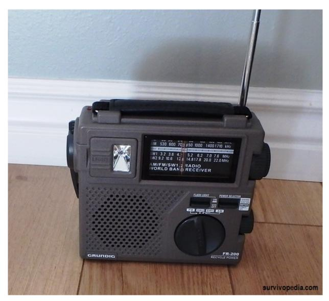
4. Wrap the third radio in a non-conductive envelope and store it (turned off) in a Faraday cage.
