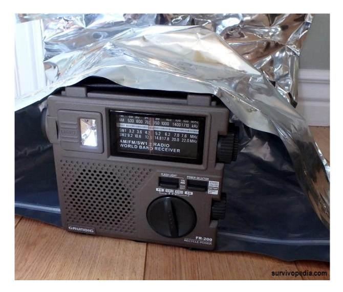
After the power goes out, check the first radio. If you hear your local radio station, the outage was probably not caused by an EMP or it was a very minor one.
