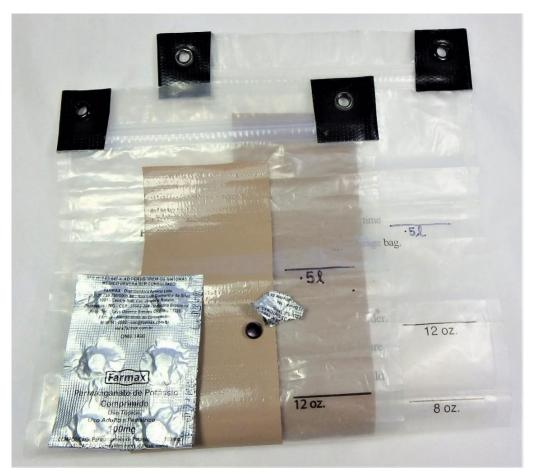
While chemical water disinfection with potassium permanganate is far from ideal (it is a poor disinfectant), long storage life, extreme multi-use, and compactness make it worthy of inclusion in pocket survival kits. A single tiny tablet can treat more water than you are likely to drink in a week-long survival ordeal. Potassium permanganate is also used to improve water quality and to oxidize iron and manganese for removal by filtration.
