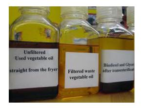
Used cooking oil has food chunks in it that need to be filtered out. Also, when you fry vegetables in the oil, water gets trapped in the oil. We can get most of that out by heating the oil gently to 70 degrees Celsius. The water will settle on the bottom and we just drain it off.
