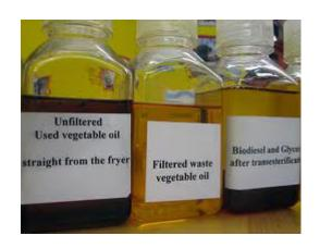
Used cooking oil has food chunks in it that need to be filtered out. Also, when you fry vegetables in the oil, water gets trapped in the oil. We can get most of that out by heating the oil gently to 70 degrees Celsius. The water will settle on the bottom and we just drain it off.
