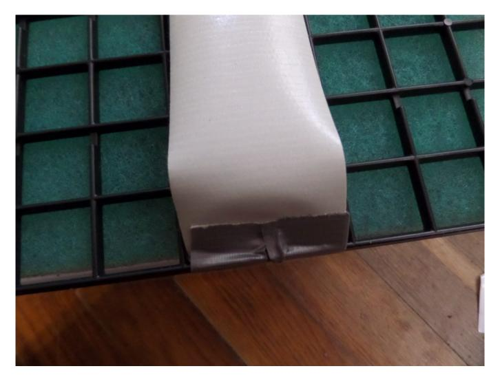
Finish off the taping by attaching it to the side of the fan. Use at least two pieces of tape for each side of the fan to ensure the filters stay in place.
