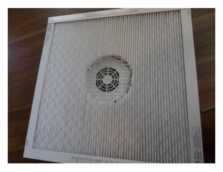
If you are using a prefilter, you will also have to cut a hole in that one. Keep the first filter in place and fit the template back over the hole. Make sure some sticky tape is exposed.
