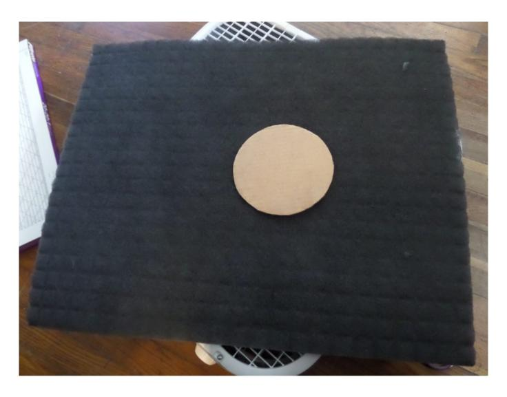
As long as the filter is not pleated, you can just use the scissors to cut around the template.
