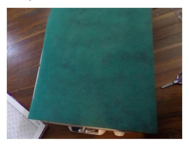
if the filter is too large in length or width, use the scissors to cut it down to size.
