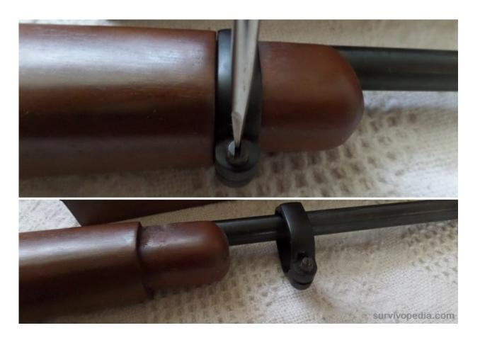
**Step 4** — Loosen barrel stock screw.
