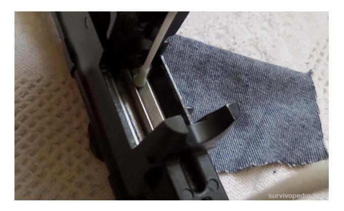
**Step 11** — Use gun lubricant to lube the receiver and trigger cross pins, various pivot points in the trigger guard housing (such as the trigger pivot, hammer pivot, safety, and the bolt and bolt handle.)
