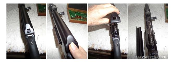
**Step 4** — Remove the recoil guide and spring. With the receiver cover off, grip the end of the recoil guide and spring unit, then push it forward until it clears the slot in the receiver. Lift it up slightly and pull it straight back out of the bolt carrier.
