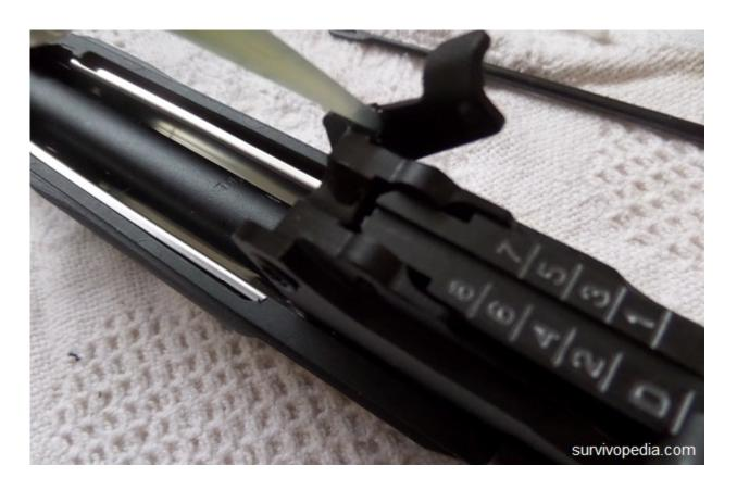
**Step 16** — To re-install the gas tube/hand guard put the front of the gas tube/hand guard into the gas tube and then push the rear section in the lock down portion in front of the rear sights. Push the take down lever counterclockwise till it locks in place in the dimple.
