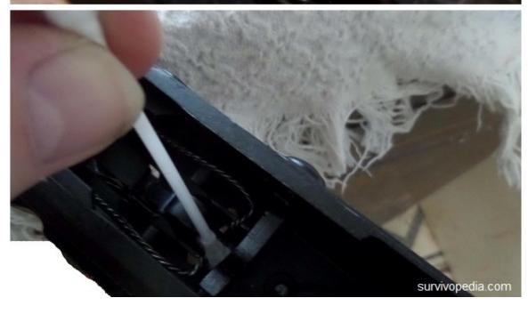
**Step 14** — Clean the gas tube using a Q-Tip with bore cleaner and clean the gas tube area. If the gas tube holes are blocked, use a small diameter nail or a gas tube cleaning tool to remove fouling in the gas tube.
