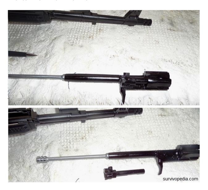
**Step 7** — Remove the gas tube/ hand guard assembly. Rotate the gas tube take down lever clockwise to about 11 o'clock position. Then lift up on the rear of the hand guard and pull it back and out of the AK gas tube.
