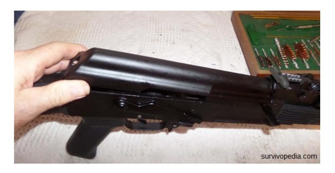
**Step 24** — Function test the AK by pulling the charging handle back and letting it go to cock the hammer. Then pull the trigger to drop the hammer. Do this 3-4 times to verify that the AK is working correctly.
