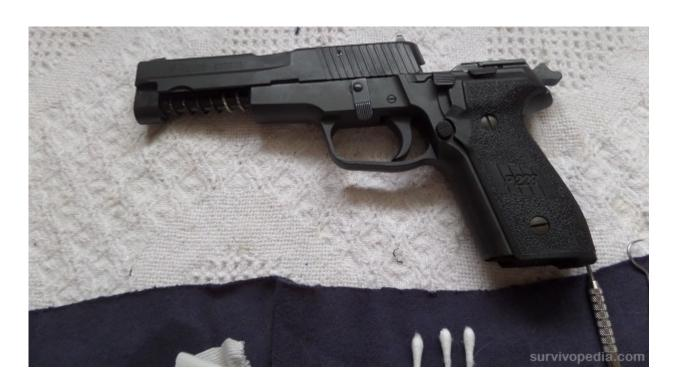
Step 5- The slide consists of 4 parts: the barrel, recoil spring, guide rod, and the bolt assembly.
