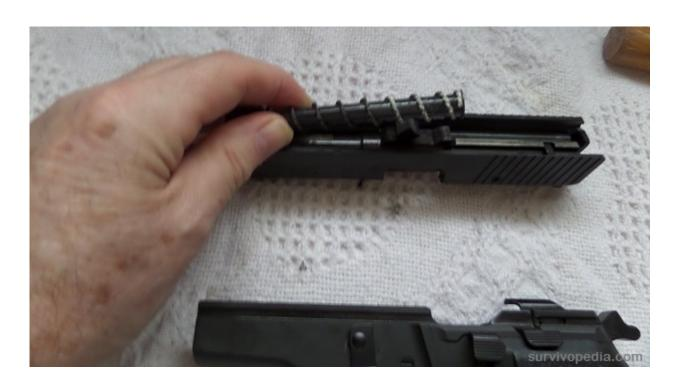
Step 7- Once the guide rod and spring are out of the slide it is easy to remove the barrel. This is done by gently pulling the barrel back about an inch. Then lifting upwards and backwards to remove the barrel from the slide.
