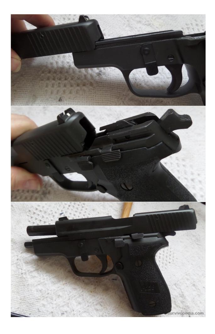
Step 28- Push the take down lever counter clockwise from the 6 o'clock position to the 3 o'clock position to lock the slide on the frame. Function test the pistol for proper functioning.
