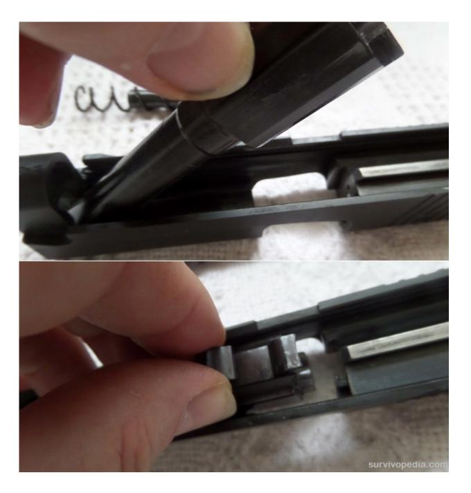
Step 26- Next place the spring and guide rod assembly in the front of the slide in the upper hole with the excess spring side of the assembly going in first. Then compress the spring with the guide rod and place it in the guide rod holding section of the barrel.
