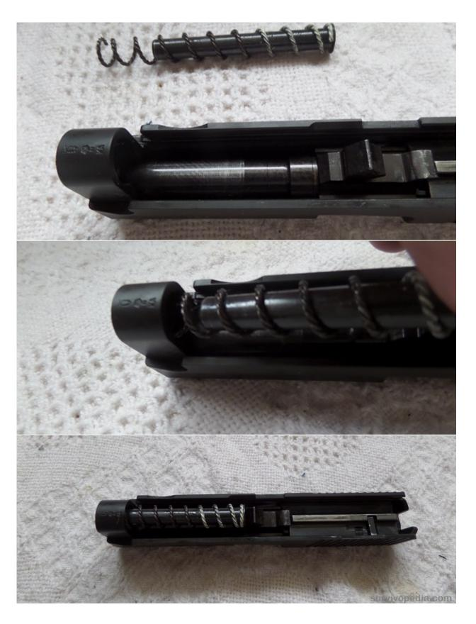
Step 27- Reassembling the slide to the frame is done by putting the rear of the slide rail groves on to the slide rails of the frame. Continue pushing the slide up the rails until the slide is all the way back and can be held in place there with the slide release.
