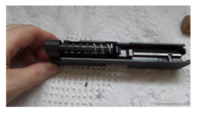
Step 6- To remove the recoil spring and guide rod from the slide, push the guide rod forward into the slide and lift off the spring and guide rod as a unit. Be careful, because this this assembly can easily slip from your fingers and fly away from you. If it hits you in the eye it may cause an eye injury.
