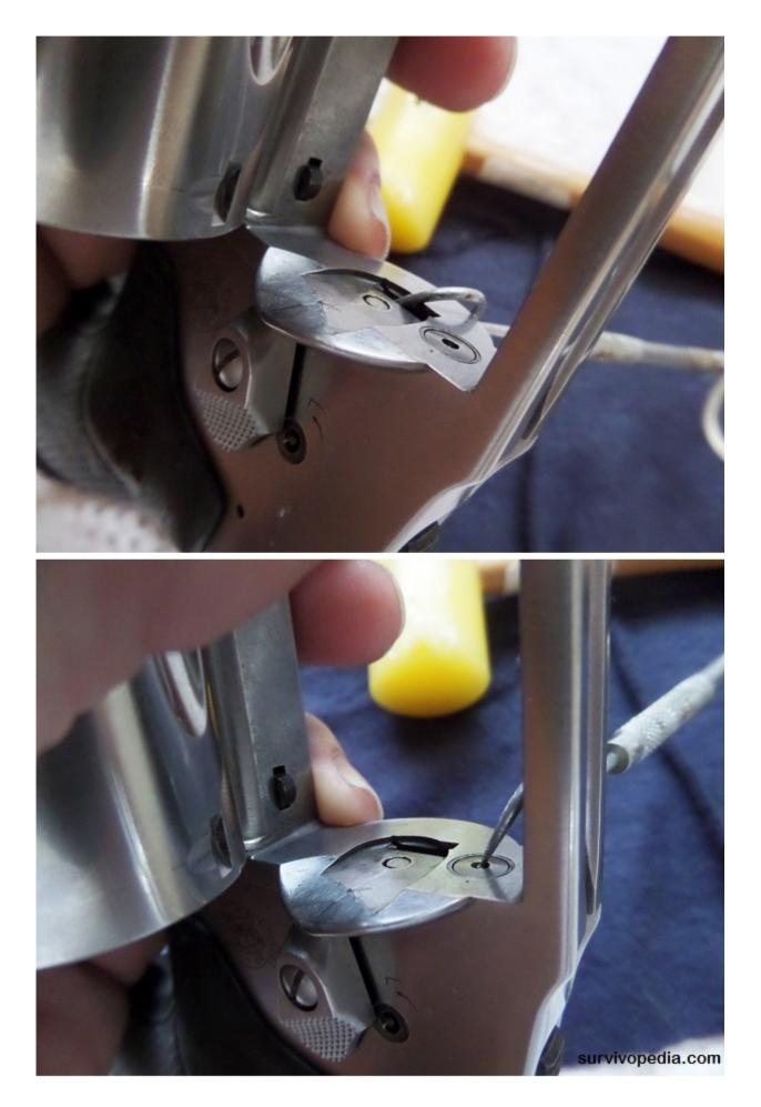
Step 8 – Use a small metal pick to remove dirt, grime, or
