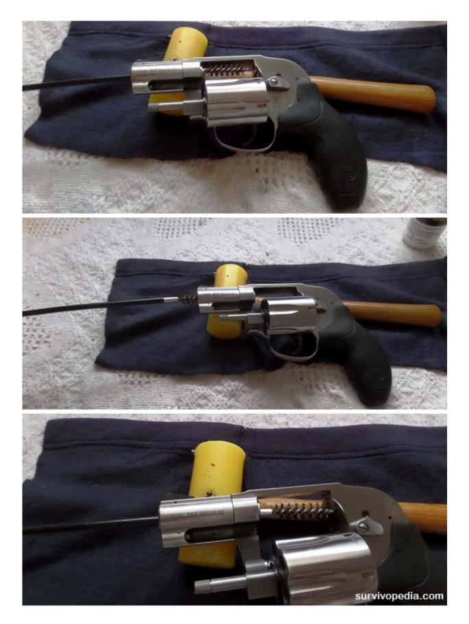
**Step 4** – Remove the cleaning brush from the cleaning rod and replace it with the cleaning patch tip on the cleaning rod. Put a clean lubricated patch through the patch tip. Insert the cleaning rod down the barrel from the muzzle end.
