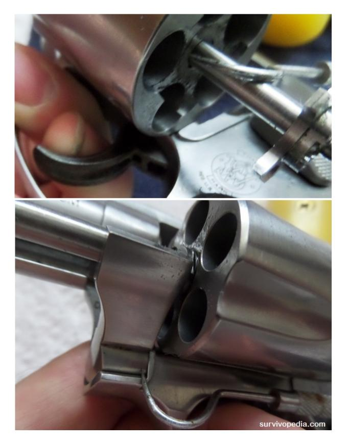
**Step 9** – Lubricate the lock works with a good quality firearms lubricate.
