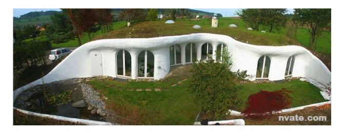
The home would stay cool in the summer, because of being underground and remain warmer in the winter, due to its ability to keep from losing heat. The ground around and over the home would act as excellent insulation to help the home maintain a comfortable temperature, year round.
