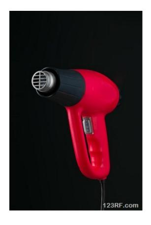
The best way to use the heat gun is to go back and forth over an area and then wipe off with paper towels or rags. The heat gun method can also be used on metal parts by going back and forth over the cleaning area.
