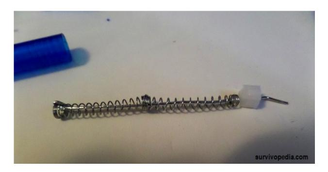
Step 9: Turn the push button so that the narrower portion is facing the spring assembly. Make sure that you are using the end that easily slides into the pen.
