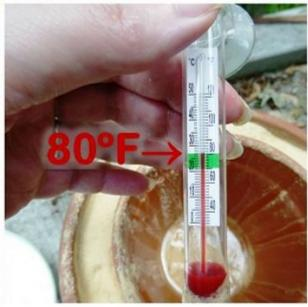
The termomether is indicating temperature after sitting inside the cooler for two hours.
