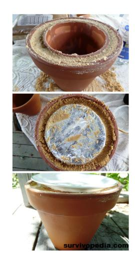
Once you reach the top, leave approximately one inch below the top of the pots so that you have a small channel for adding water later on.
