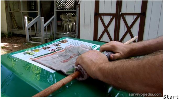
the paper near one end of the dowel so that it is easier to push off once you are done rolling paper. As you roll the newspaper squeeze out excess water.
