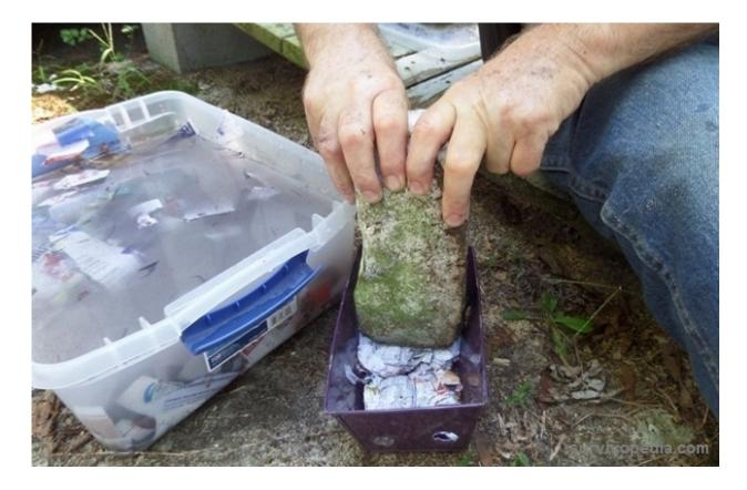
Turn the sieve pan upside down and tap on the bottom of the sieve pan to release the paper brick. Let small bricks dry in the same way as paper logs and larger bricks.
