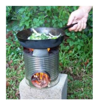
A rocket stove uses a small wood fire to heat a combustion chamber so that your fuel is used efficiently.
