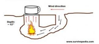
A Dakota Fire Pit is use to burn safely underground. To make this fire pit, dig two vertical shafts which are connected by a tunnel.
