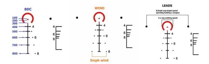
The horseshoe reticle allows for fast target acquisition within 300 meters. The two dots on either side of it are used as leads for an 8.6 mph running speed.
