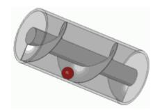
Essentially, this is a "screw" shape housed inside of a round tube. As the screw turns, it draws water upward despite the effects of gravity.
