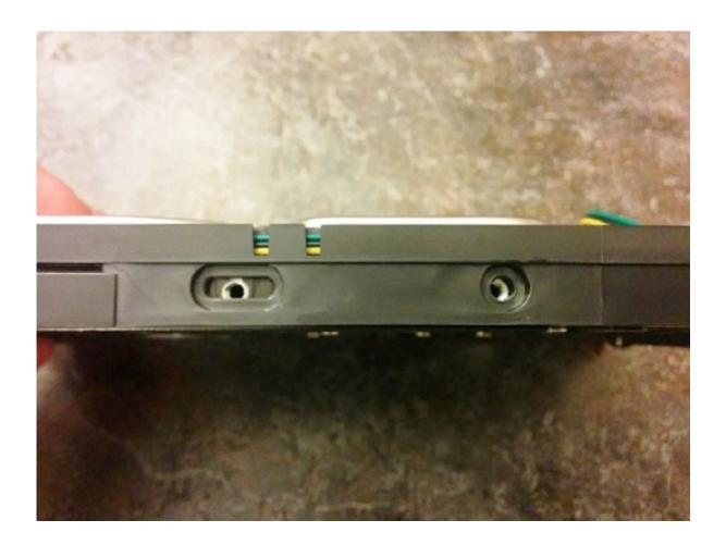
**Step 6** — Secure the hard drive to the plastic slide. Each side should have 2 screws. Make sure that the connections are still secure while you do this.
