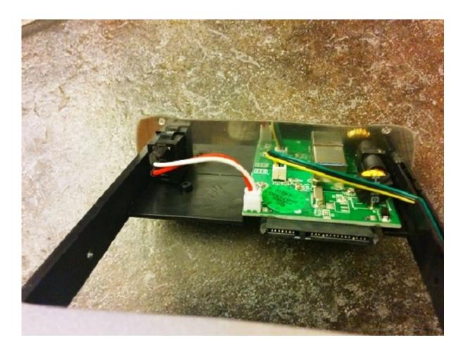
Notice the connections on the enclosure. You will want to line these up with the connections on the hard drive.
