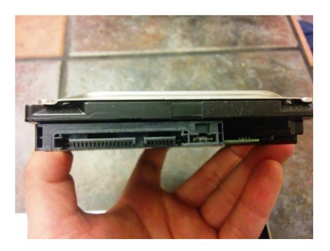
Step 4 — Identify the type of hard drive you have. The hard drive above is an SATA hard drive. It is a more modern hard drive compared to and IDE hard drive. The documentation on the top of the hard drive would also tell you what kind of drive it is and the capacity. This hard drive is 500 gigs. That's a lot of preparedness resources!!! For a video tutorial on identifying hard drives — click here.
