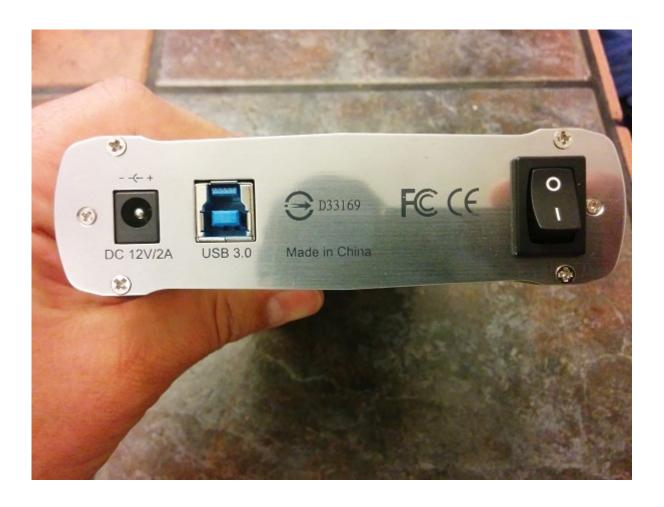
**Step 7** — Secure the plastic slide to the outside enclosure by screwing in the 4 small screws.
