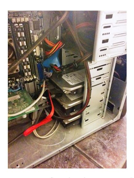
Step 2 — Unplug the wires connected to the hard drive. You might have to remove plugs on the motherboard too. If you think you might get this computer fixed at some point, make a note of where those plugs are connected. If you are going to donate the parts or chunk the rest, then don't worry about it. NOTE: It is a good practice to ground yourself when working inside your computer. Simply make sure you are touching a metal portion of the computer enclosure.
