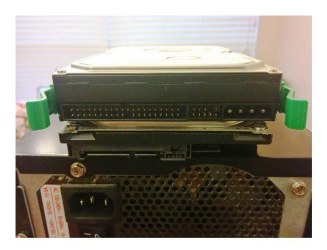
The pic above is of two hard drives stacked on top of each other. The one on top, with the green slides, is an older IDE hard drive. The one below is the SATA hard drive that I just removed from my computer. This is important to know because you need to match the type of enclosure with the type of hard drive you have.
