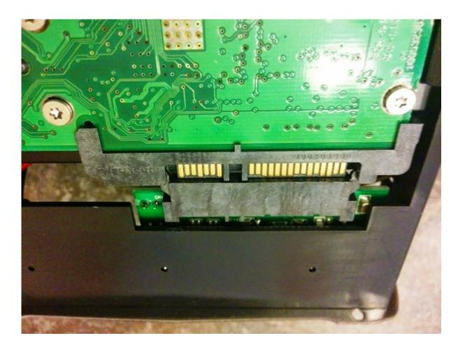
Here is a pic of the hard drive and enclosure being connected. Notice that this one will snap when it is completely secured. Don't force this. If you damage the connection, you might ruin your hard drive.
