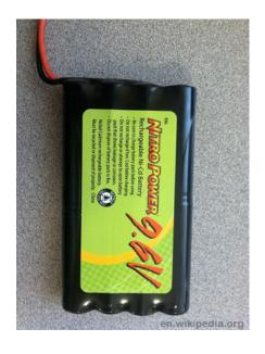
They differ from other batteries in terms of their ability to deliver a steady charge even if the are almost out of power.
