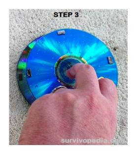
Step 3: The magnets should attract to the ones on the other CD and hold the two disks together. For this demo, I did not glue the disks together, however that would be necessary for units that will turn at a higher RPM.
