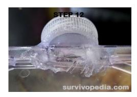
Step 12: Seal the outer edges of the CD to prevent air or water from escaping.
