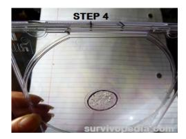
Step 4: On the lid of the jewel case, draw a box that will be cut away to make an opening port for the turbine.
