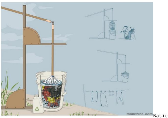
ally, this highly portable muscle-operated washing machine is made of three main components: the container itself, a net bag (this is designed to agitate the clothes while it holds/squeezes them) and the mechanism itself, which is a lever-driven shaft kept together by a wooden frame.
