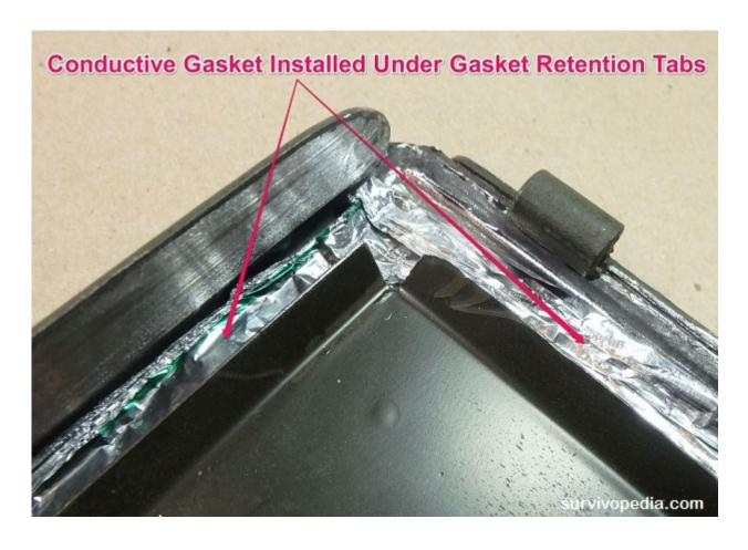
Maybe I'll build some ammo can Faraday cages for radio and battery kits with conductive gaskets but since most of you will use tin foil, I will demonstrate the technique in this build.
