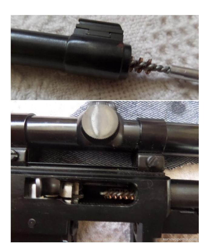
**Step 8** — Remove the bore brush from the cleaning rod and replace it with the patch tip. Then place a clean dry patch on the tip and run it down the barrel from the muzzle to the receiver. At the receiver replace the dirty patch with a clean one and pull it back through the barrel and out.
