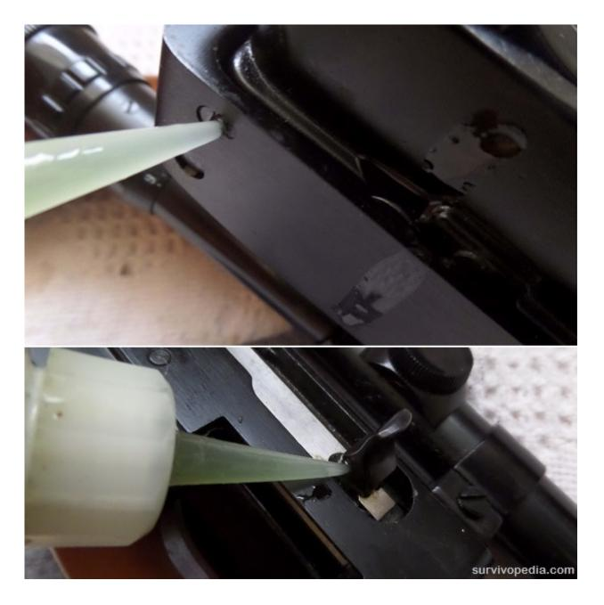
**Step 12** — Before final assembly of the barreled receiver to the stock wipe down with a good gun lubricant all the metal parts that will be contained within the stock and outside of the stock.
