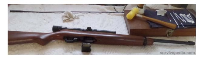
${f Step~3}$  — Loosen the front band screw and remove the front band.
