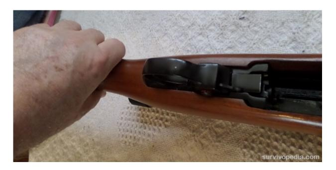
**Step 6** — Swing the barrel and receiver mechanism upward and away from the fore-end.
