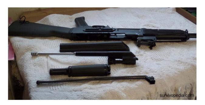
**Step 9** — To clean the barrel use a bore brush of the correct bore diameter and soak it with bore cleaner. Push the brush 8-10 times through the barrel going from the chamber to the muzzle. Remember to remove the wire brush each time before you pull the cleaning rod back to to the chamber and re-install the wire brush For the next push of the cleaning rod.
