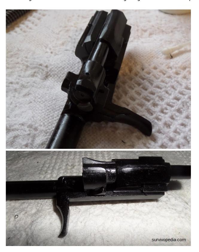
Step 20 — Insert the bolt carrier assembly into the gas tube.
