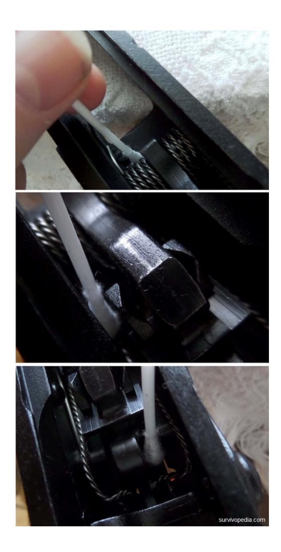
**Step 13**— Use gun lubricant lightly to lube all of the receiver components.
