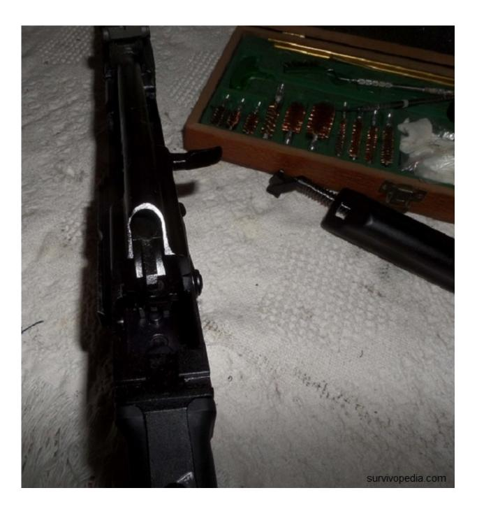
**Step 22** — To re-install the recoil guide and spring unit, push it forward into the back of the bolt carrier assembly until it clears it's slot in the receiver. With your fingers, ease it back until it locks into the slot.
