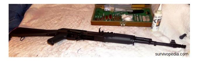
**Step 3** — To begin breaking down the AK, first start by removing the receiver cover. To do this hold the rifle butt stock firmly in one hand. Then with the thumb of the other hand push forward on the end of the recoil guide and lift the receiver cover upward and back from the receiver.
