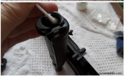
**Step 15** — Put a drop of lubricant on the gas tube take down lever.
