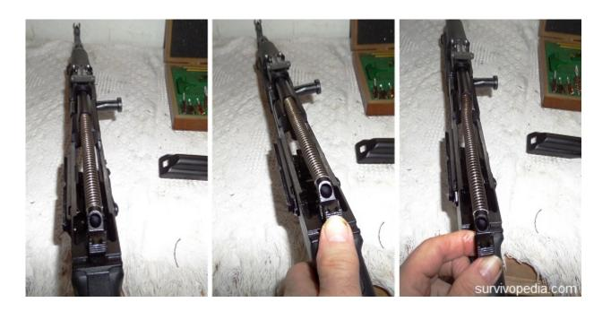
**Step 5** — Remove the bolt carrier assembly. Ensure that the safety is in the FIRE position. Grasp the bolt handle and pull it back to the full rear of travel. Lift the bolt carrier assembly up from the receiver and draw it to the rear and out of the gas tube/hand guard assembly.
