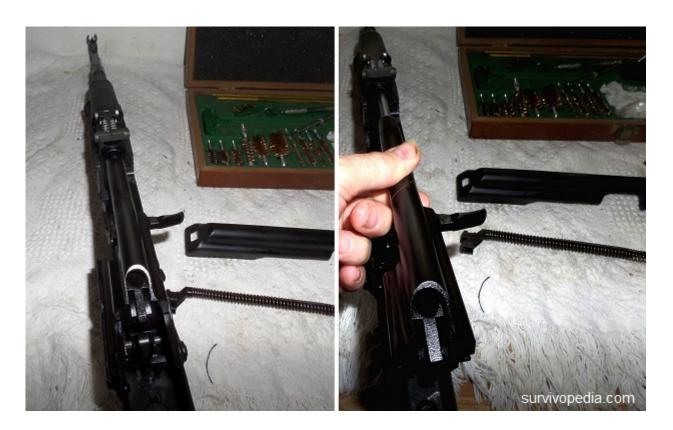
**Step 6** — Remove the bolt head from the carrier assembly hold the carrier in one hand. Then with the other hand rotate the bolt head out of the locking groove. Pull the bolt head out of
