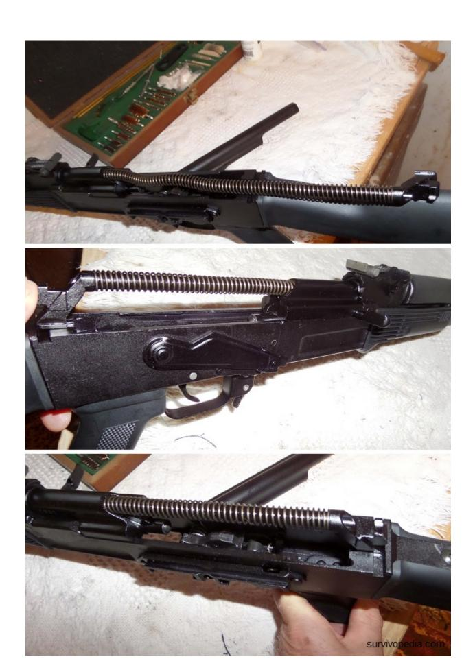
**Step 23** — To re-install the receiver cover, put the front of the receiver cover into the slot behind the front sight. Push
