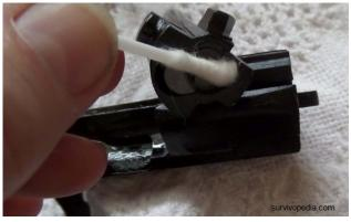
**Step 19** — To remount the bolt face shaft into the bolt, push the bolt face and shaft into the bolt until the locking lug lines up with the groove in the carrier assembly. Twist the bolt face shaft clockwise to engage the groove. Continue twisting the shaft until the locking lug is locked in place.
