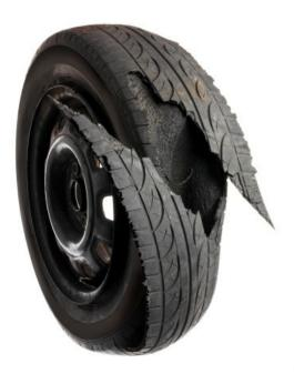
Most of us try to keep good rubber on our vehicles, changing the tires when they start going bald. But every once in a while, we miss the signs, especially for the tires on a trailer that has been sitting for a while. The rubber in the tires may be dry, allowing it to wear off excessively rapidly and leaving us running on a tire with the belts showing through.
