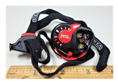
The Petzl e+Lite is a very small purpose-designed emergency headlamp. It is very compact and runs on two CR-2032 lithium coin cells which give it a burn time of nine hours at 50 lumens, twelve hours at fifteen lumens. This headlamp also has a two-lumen red LED and strobe settings for both white and red LEDs. The e+Lite is well designed, and the on/off switch features a lock position, so it is unlikely that it will get turned on inside a kit.
