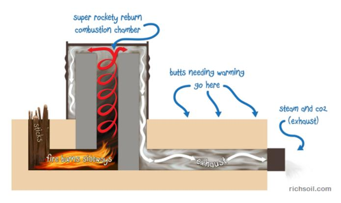
After the wood is burned with great efficiency at high temperatures thanks to the insulated combustion chamber (the heat riser), the exhaust gases pass through a large thermal mass (usually made of cob but it can be anything, such as brick, stone, tile or masonry) that absorbs the heat before the gases escape outside.
