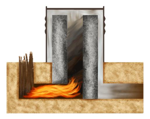
Basically, an RMH is a high performance, clean, highly efficient wood burner that can be built using recycled materials and/or natural materials like cob. You don't have to be a professional and you don't need complex masonry skills. This is a basic DIY job for the average Joe, any day of the week.
