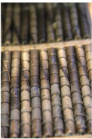
When it comes to off grid survival, there are only two advantages to using an Edison Battery. First, these are the only rechargeable batteries that can withstand recharging on a daily basis. In fact, many people today that generate power from windmills rely on Edison Batteries because they do not break down for years on end.
