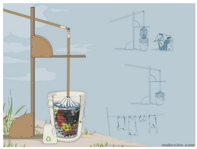
Basically, this highly portable muscle-operated washing machine is made of three main components: the container itself, a net bag (this is designed to agitate the clothes while it holds/squeezes them) and the mechanism itself, which is a lever-driven shaft kept together by a wooden frame.
