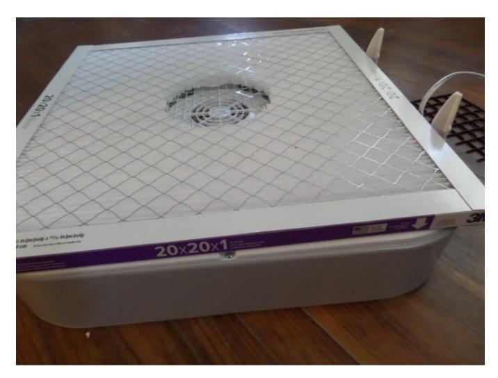
Place outer filter on top so that the holes line up with the holes in the fan motor.
