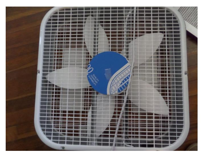
Lay the innermost filter on top of the fan and template. Make sure that the air flow arrows on the filter match the direction the air will flow through the fan. Press down slightly on the center of the filter. At this point, the template should stick to the filter. Simply lift the filter up and you will know exactly where to cut the hole into the filter.
